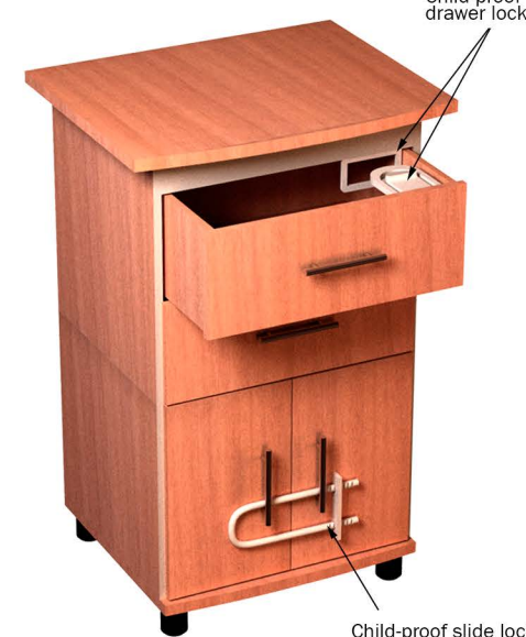
Figure E. Securing cabinet doors and drawers.
