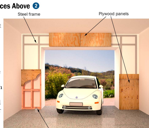
Figure B. Strengthening garage walls below living space.
